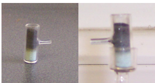
Figure 58: Pictures of the copper oxalate residue observed after heating in the large volume removable cell placed in the cup stalk.
