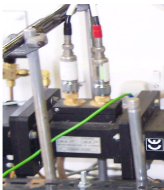
Figure 17: Picture of the microwave power meter
