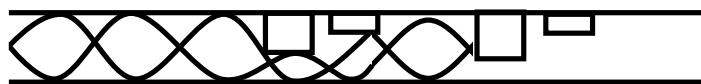
Figure 27: Fundamental diagram of the returning wave reflecting off the second set of stubs
