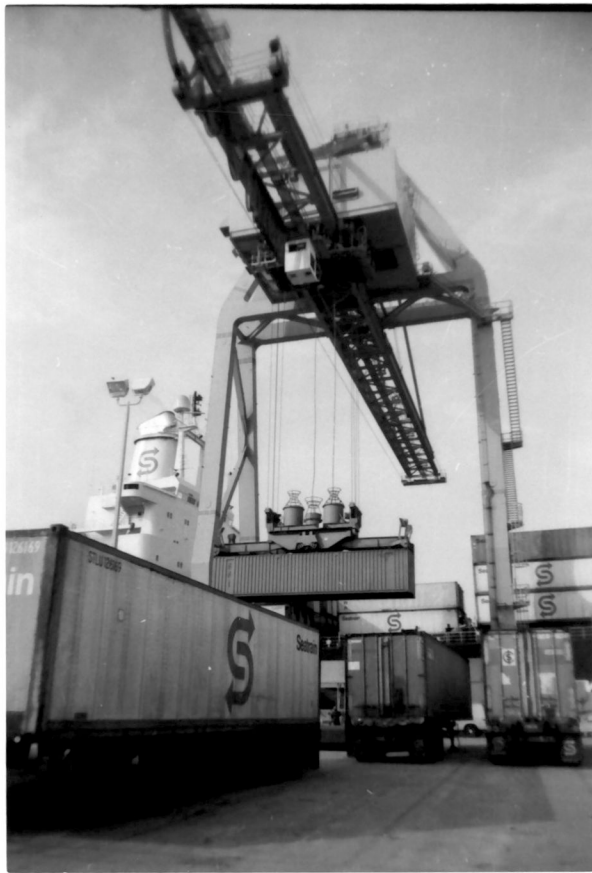
Figure 11: Container crane unloading containers onto truck bodies for transshipment.
