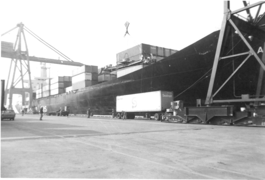
Figure 8: Special adapter that enables gantry cranes to load and unload containerized cargo.
