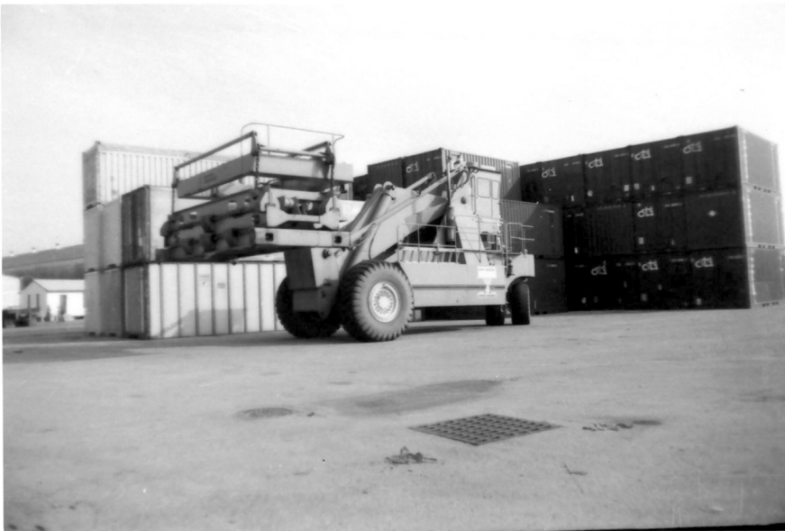
Figure 9: Specialized piece of equipment utilized for stacking containers in storage areas.
