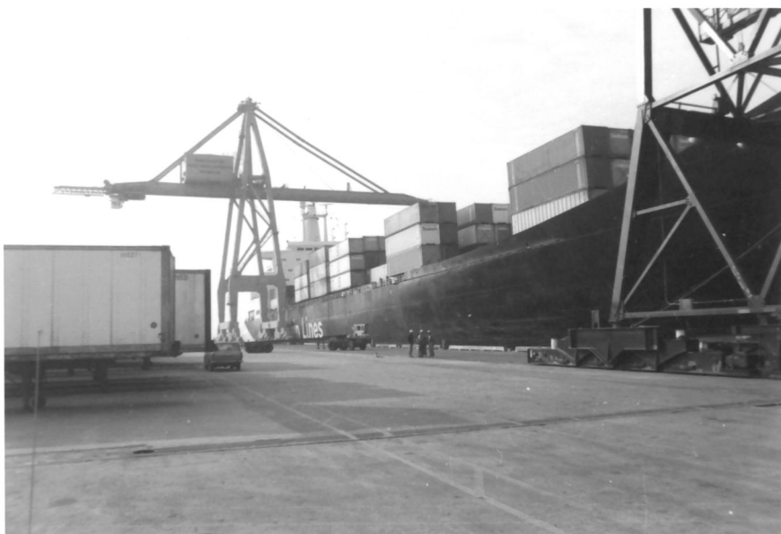
Figure 6: Container crane unloading the middle section of a container ship at the Wilmington port.
