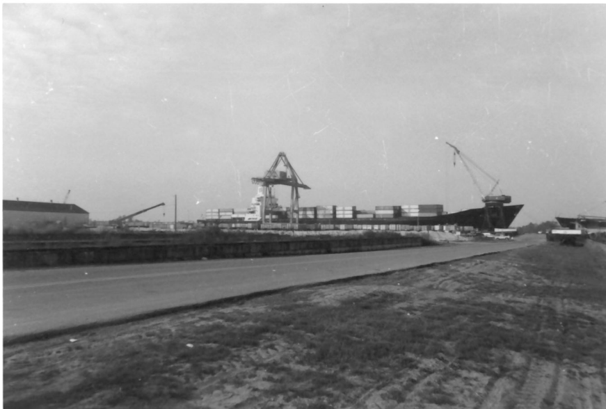
Figure 5: Simultaneous unloading of a container ship at the Wilmington port by a container crane and a gantry crane with an adapter for container handling.
