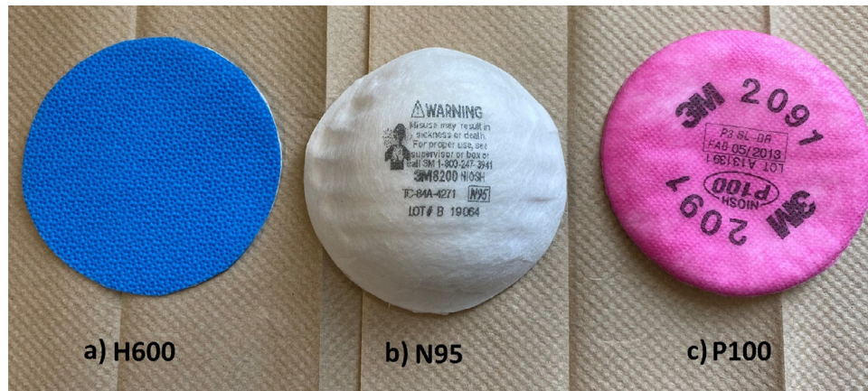
Fig. 1. Four-inch Diameter Test Filters: (A) Halyard H600, (B) N95, (C) P100.
