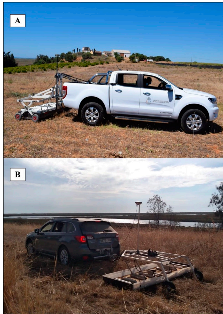
Figure 3. The GPR equipment used: (A) GPR Stream X; (B) GPR MkIV.
