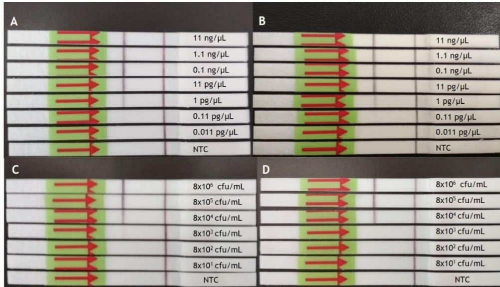
Figure 5.9. Results of the analytical sensitivity for L. monocytogenes detection for RPA-LF reaction. (A) and (B) show the lowest concentration of DNA possible to detect with qPCR and RPA primers, respectively. (C) and (D) present the results of the lowest bacteria concentration detected by RPA-LF using qPCR and RPA primers, respectively. NTC correspond to the “no template control”
