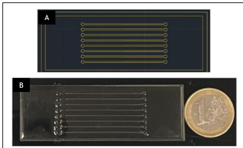
Figure 3.2. Microfluidic PDMS device with 8 capillarity-driven microchannels to performed DNA amplification (PDMS channels prototype). (A) Design in AutoCad and (B) PDMS replica after fabrication
