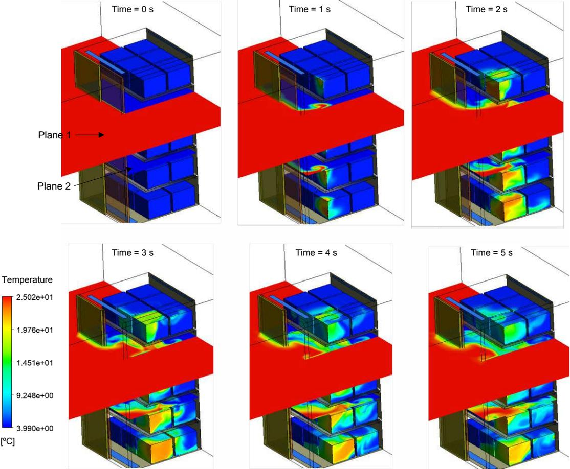
Figure 2. Temperature distributions inside the cabinet and over the products from instants 0 to 5 seconds.
