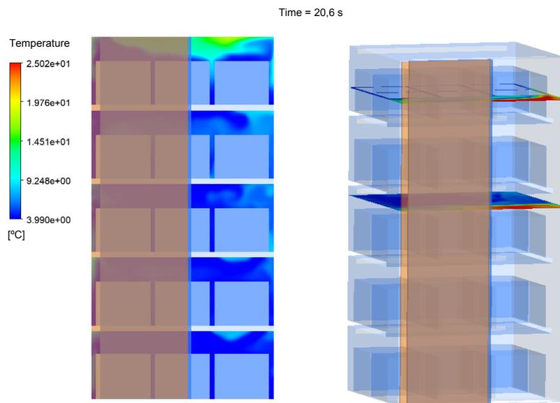
Figure 5. Temperature distributions in different planes inside the cabinet at instant 20.6 seconds.
