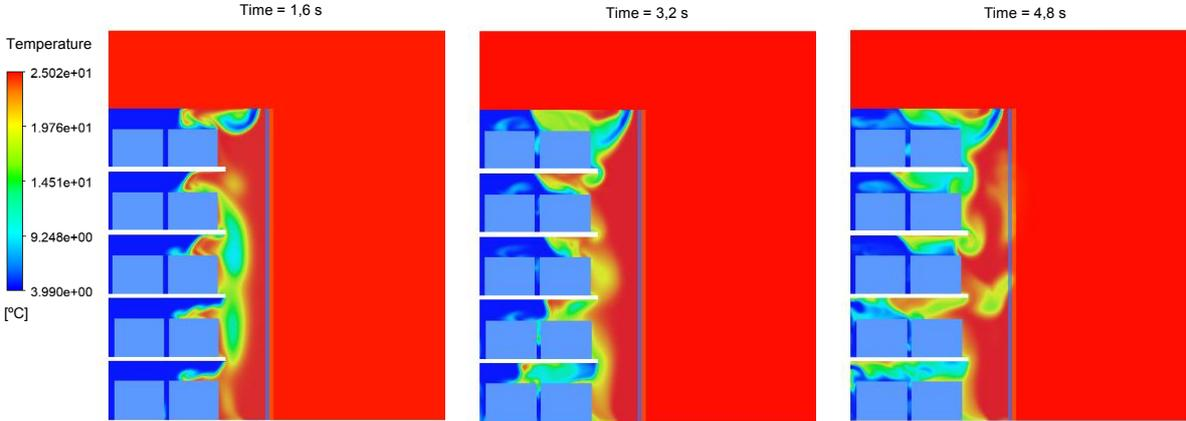
Figure 3. Temperature distributions along the air curtain and inside the cabinet from instants 0 to 5 seconds.
