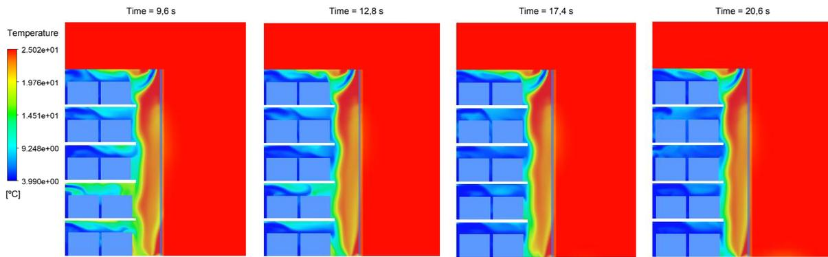
Figure 4. Temperature distributions along the air curtain and inside the cabinet from instants 9.5 to 20.5 seconds.
