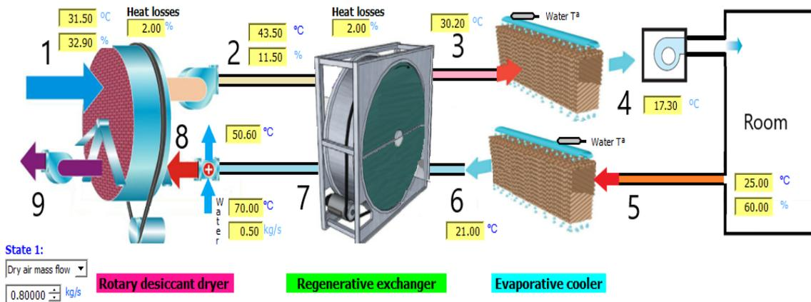
Figure 2. Pennington cycle (ventilation cycle).
