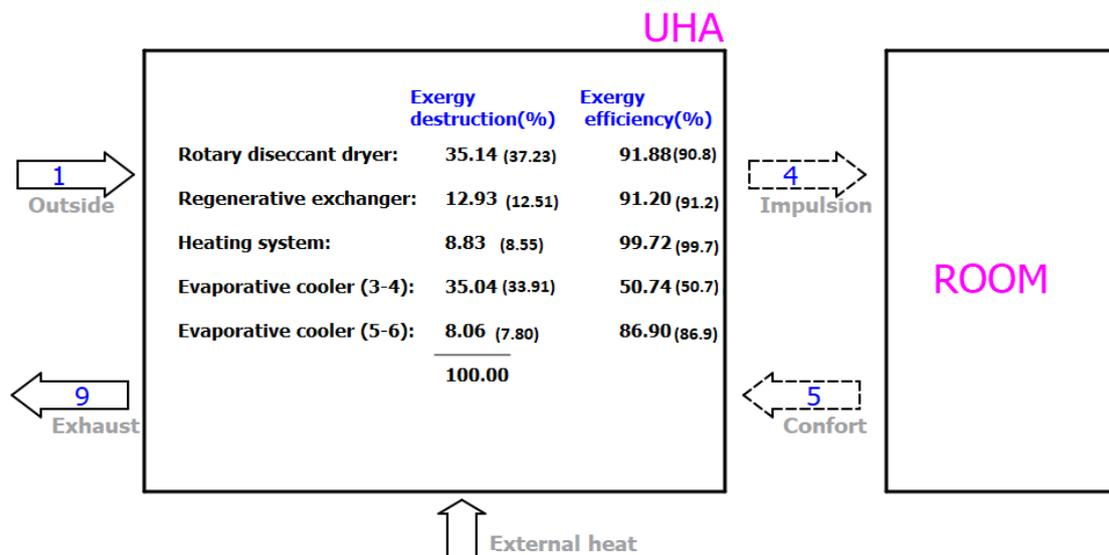
Figure 8. Summary of exergy destruction in the elements of the installation.
