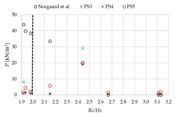
**Figure 7.** Horizontal pressure calculated by Nørgaard et al. (2013) [15] and measured at sensors PS3 to PS5.
