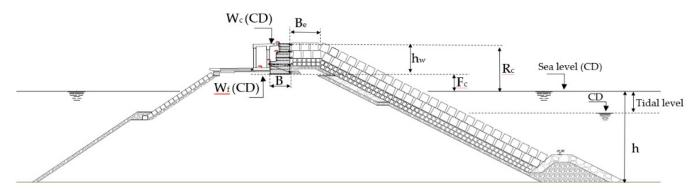
Figure 3. Main parameters of the cross section.
