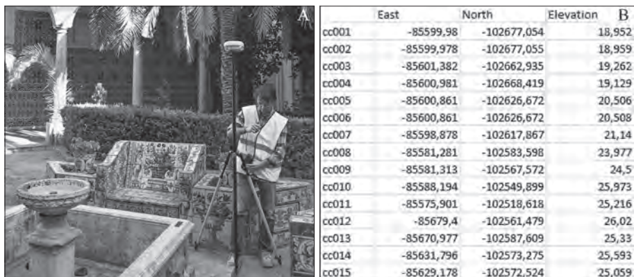
Fig 9. (A) Trimble R8 GPS Receiver; (B) 14 Coordinate Point.
