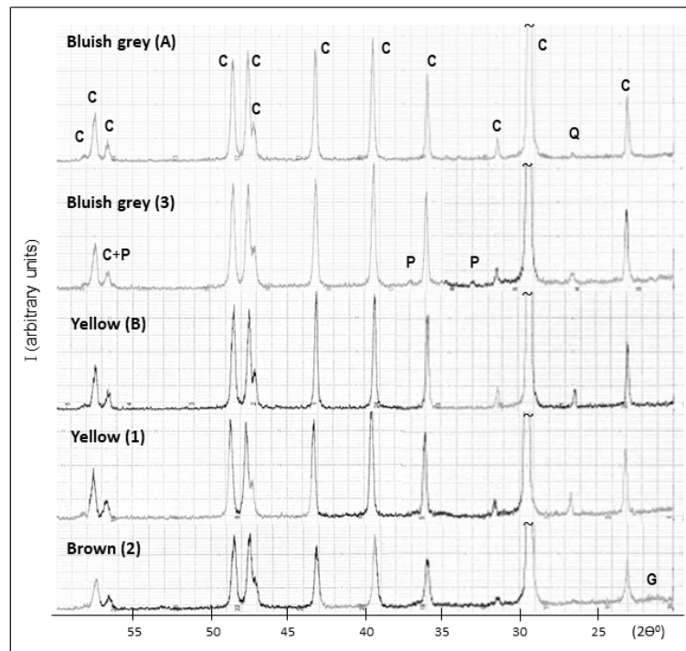
Figure 11. XRD patterns of Azul Valverde bluish-grey, yellow and brown uneven fragments; C—Calcite, \text{CaCO}_3 (JCPDS card number: 5-0586), G—Goethite, \alpha\text{-FeO(OH)} (17-536), P—Pyrite, \text{FeS}_2 (6-0710); Q—Quartz, \alpha\text{-SiO}_2 (5-0490).
