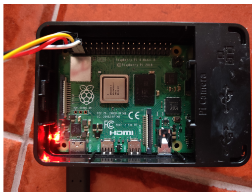
Figure 5.1: Connections to Raspberry Pi
