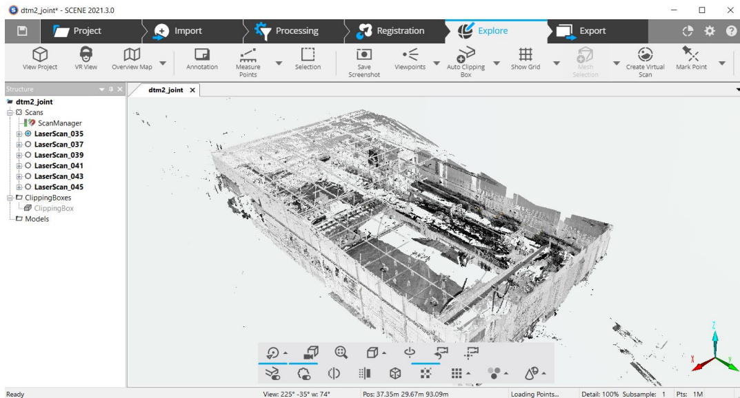
Figure 65 - Point cloud in the SCENE software.
