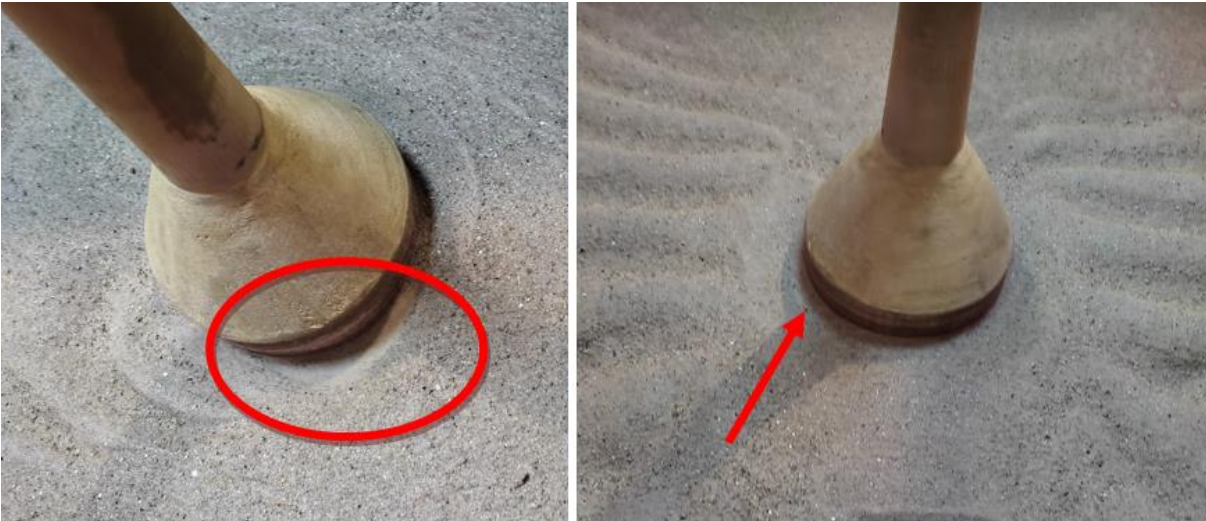
Figure 94 - Layered sand scour hole "Waves2" (Left); and "WEC4" (Right).
