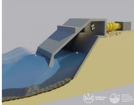
Figure 23 - Oscillating water column (MOREnergy lab, 2022).
