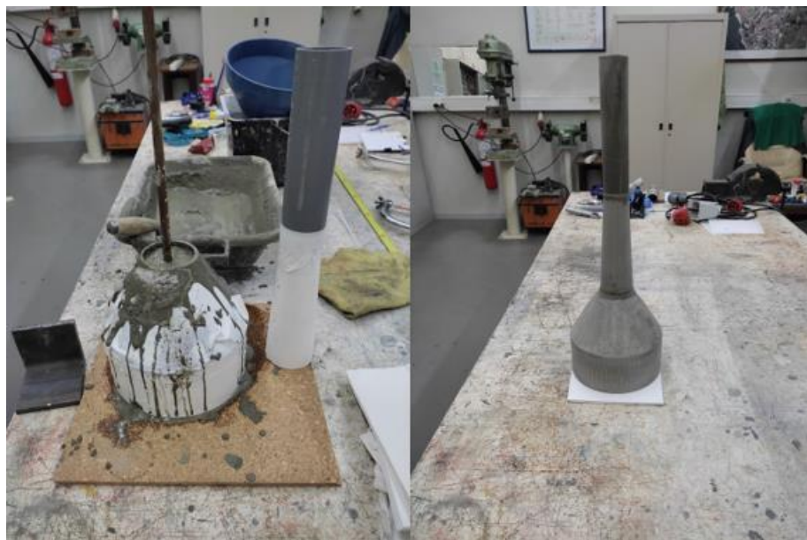
Figure 38 - Outside mold (left); and final concrete GBF model (right).
