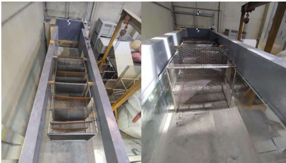
Figure 49 - Dissipation system fixed to the flume.
