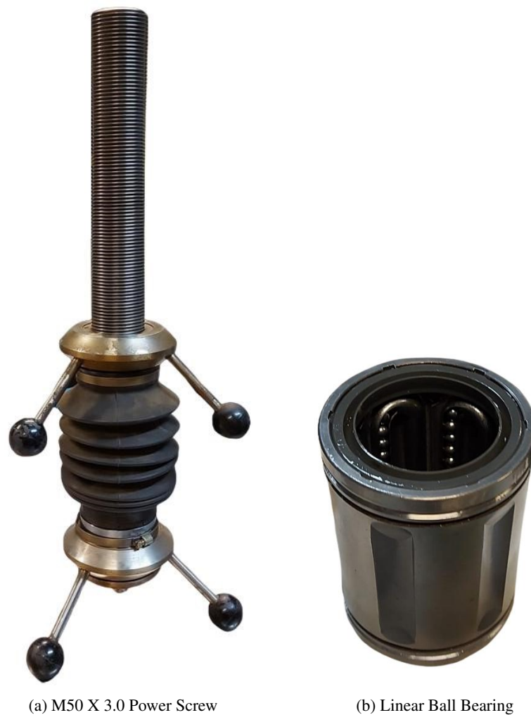
Figure 3.2: Power Screw and Linear Ball Bearing existing in the original structure
