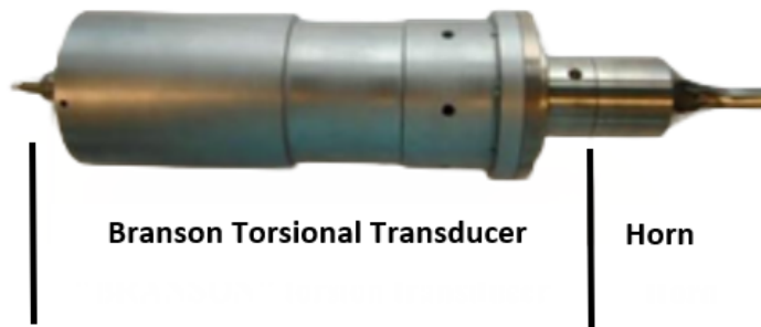
Figure 2.13: Torsional piezoelectric transducer, ultrasonic horn and specimen (Adapted from [12])
