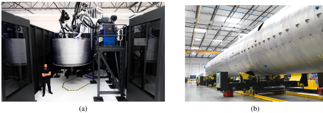
Figure 2.13: Relativity - 3D printed rocket: (a) Stargate; (b) Rocket structure [22].
