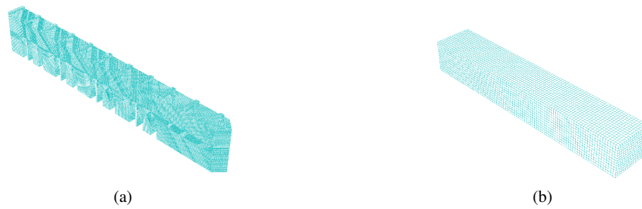
Figure 3.7: Benchmark Bridge Mesh: (a) Bridge (b) Substrate.
