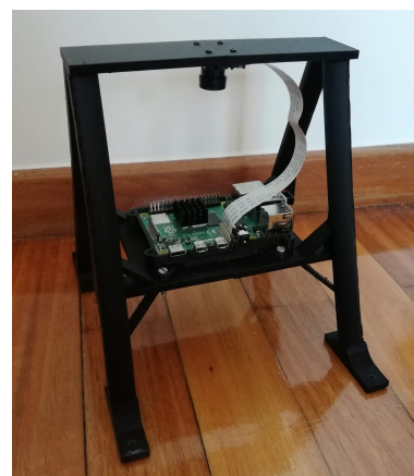
(c) Support 3D printed. with camera and RPi installed
