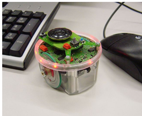
Figure 2.5: The e-puck robot with the basic extension board [2]
