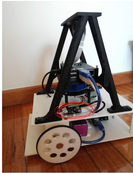
Figure 4.9: New location of the LiDAR board
