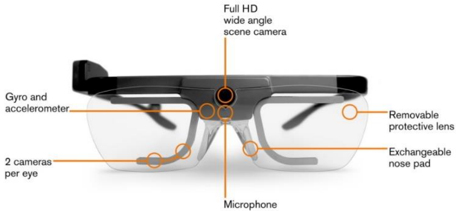
Figure 9.2: Structure of an eye tracker (Source: tobii.com)
