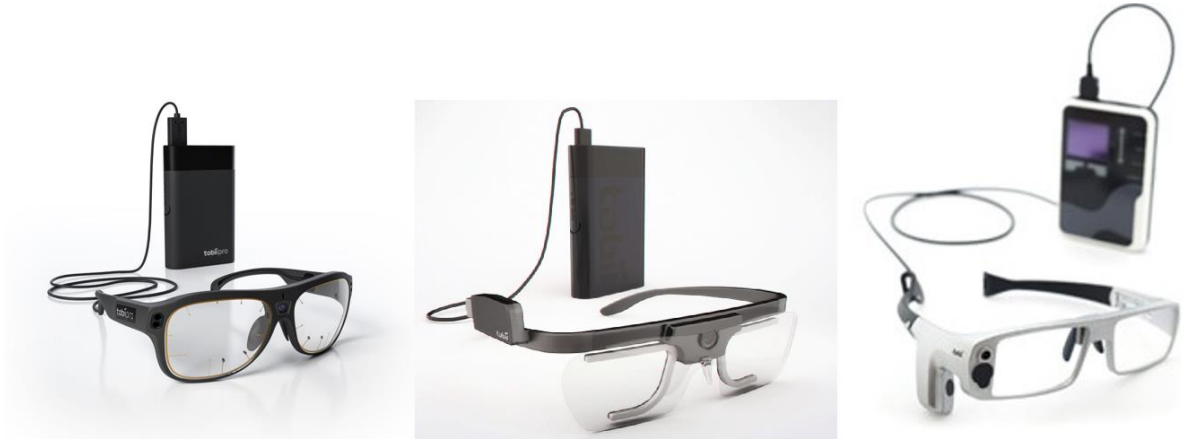
Figure 9.1: Three generations of Tobii Glasses mobile eye tracker (Source: tobii.com)
