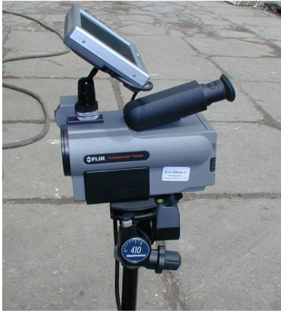
Thermovision camera used for the survey
