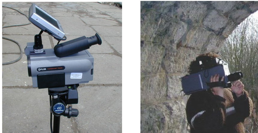
Fig. 1. Instrumentation of infrared thermography. FLIR system (left), AGEMA system (right)
