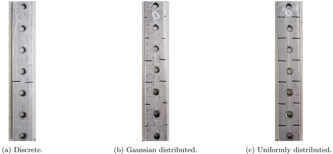
Figure 4: Photographs of the three differently damaged fishplates.
