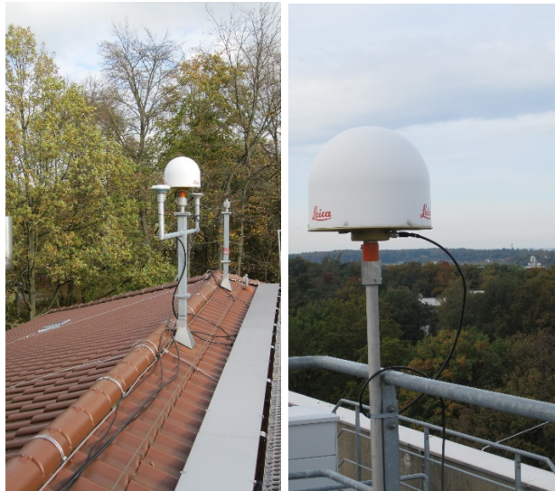
Fig. 3: Experimental setup at the PTB Campus Braunschweig, Germany. Top: google view of the scene showing the GNSS stations PTBB and KOP1 at the Kopfermann building (left) and the stations MEI1 and MEI2 at the Meitner building located about 290 m west and above the trees. Bottom zoom on the antennae installed at KOP1 and MEI2 used in this study.
