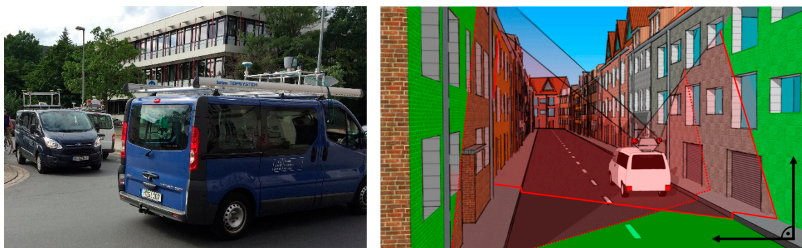
Figure 1. (left) Photograph of a typical situation during our experiments: in the first Meet and Greet scenario, all three cars meet at a junction. (right) Sensors are attached to moving sensor platforms (vehicles), i.e., sets of sensors are spatially bound to a common frame, which itself is moving through a global frame.
