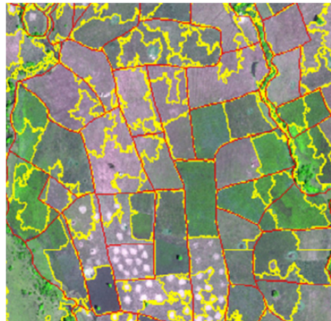
Figure 9. Wassie et al. [277] used open-source software to develop a workflow to extract smallholder parcel boundaries using HRSI in Ethiopia. Note: red = control boundaries; yellow = extracted.
