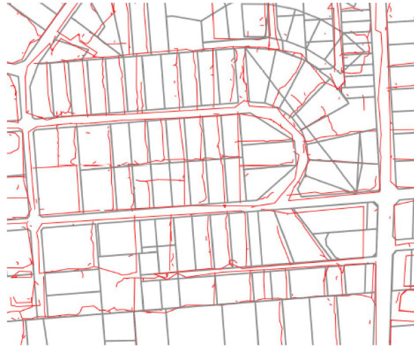
Figure 8. The 2000s saw convergence in data capture technologies and integrated workflows for map production, as demonstrated by [257], where lidar data, aerial imagery, and open-source software were used to generate a parcel layer (red lines) with limited human input. Note: grey lines are the original cadastral boundaries, used for comparison.
