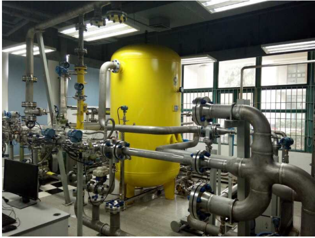
Figure 2: The pilot-scale multiphase flow testing facility at Tsinghua University multiphase flow laboratory.
