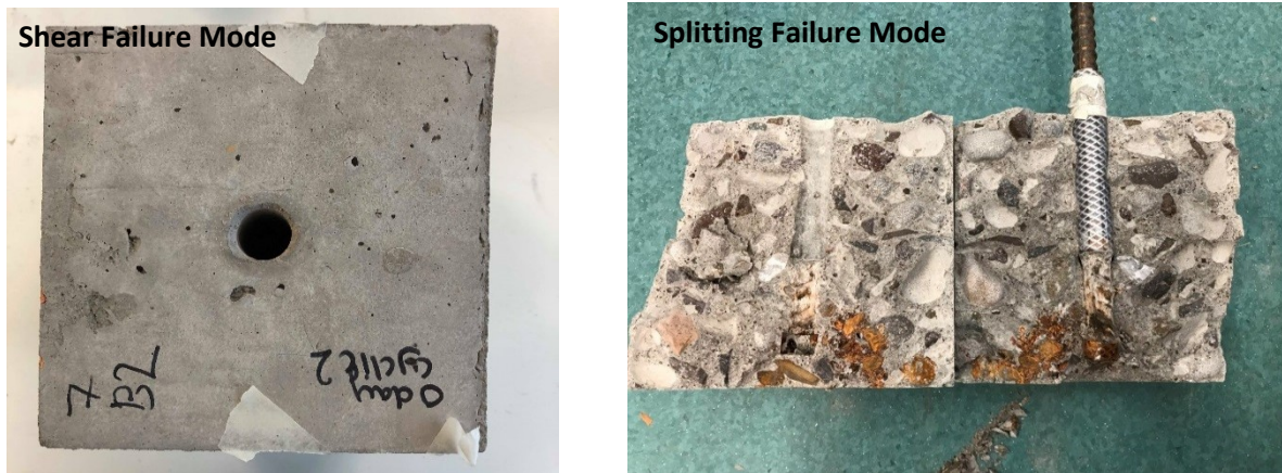
Fig 8. Specimens after Pull-out
