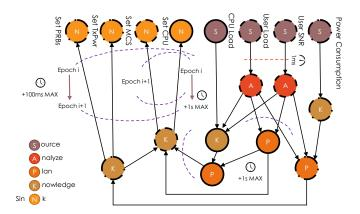
Fig. 5: The Zenoh-flow arrangement of the N-MAPE-K blocks for vrAIn and SBP-vRAN. Dashed nodes are common to both algorihtms, while solid and dot-dashed nodes are related to vrAIn and SBP-vRAN, respectively
