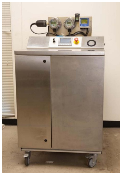
Figure 1. Shows twelve's proton exchange membrane (PEM) CO 2 electrolyzer for CO production. This system has reached the kg per day scale.
