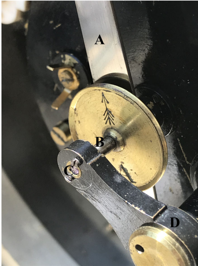
Figure 1. The magnetic needle (A) of the Royal Cornwall Polytechnic Society's Fox type, suspended by its pivots (B) between jewelled pallets. The outer jewel (C) is held within an arm, attached to an axle (D) which connects it to the circle's face. (Author's image, 2020.) (Online version in colour.)
