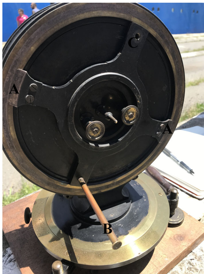
Figure 6. The reverse of the circle. A dial (A) can be moved around the circumference's vernier, adjusted in reference to the dip measured to maintain a constant difference between the needle at dip and the deflectors. The deflectors are screwed into holes. In this image, deflector 'S' (B) has been inserted, while the hole for deflector 'N' (C) is open. (Author's image, 2020.) (Online version in colour.)
