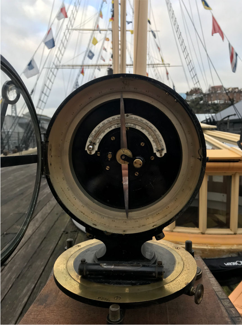
Figure 4. The Fox type on board the SS Great Britain , with the magnetic needle pulled straight down at almost 90^\circ , which erroneously indicated our position being close to the North Magnetic Pole. (Author's image, 2020.) (Online version in colour.)
