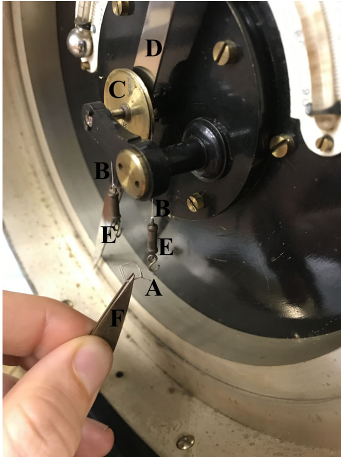
Figure 7. The performance of an intensity experiment with weights (A), underway at East London, with silk thread (B) wound around the grooved wheel (C) that is fixed to the needle (D). This thread suspends two hooks (E) to which weights are added with tweezers (F), so as to coerce the needle back to its dip. (Author's image, 2020.) (Online version in colour.)
