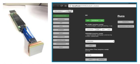
Figure 4: (a) Left panel - CHEC-S front-end electronic (FEE) module connect to each SiPM photosensor, providing full-waveform digitisation for every channel and the first-level of camera trigger, from [15]. (b) Right panel - Current camera control GUI on the GCT prototype site, with the various actions, setups and observation modes implemented.
