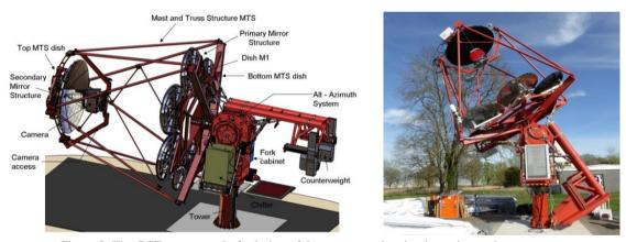
Figure 2: The GCT prototype. Left: design of the prototype showing its various sub-systems. Right: the prototype during a test in Meudon (March 2017).
