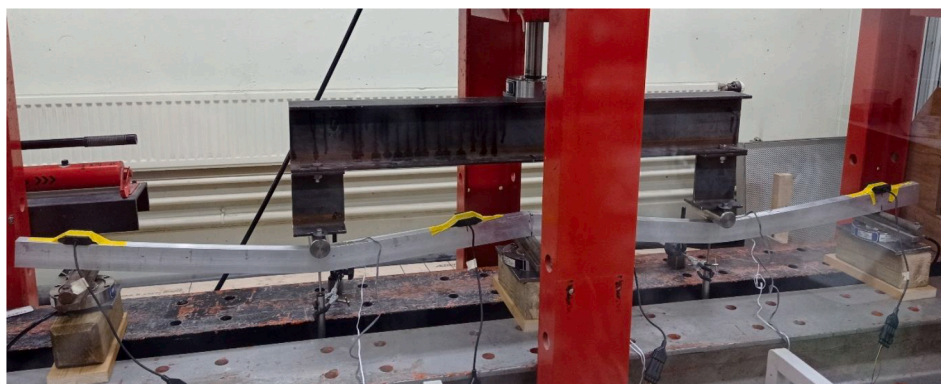
Fig. 13. Typical continuous beam test set-up.
