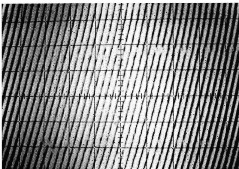
Figure 4.12 Photograph of the oscilloscope output showing the appearance of the rings from a mirror target. Both scanners are driven by triangular signals of amplitude U = 0.17 V, F_x = 20 Hz, F_y = 0.2 Hz, \delta = 3 mm, 10 mV/div horizontal and vertical oscilloscope display scale.
