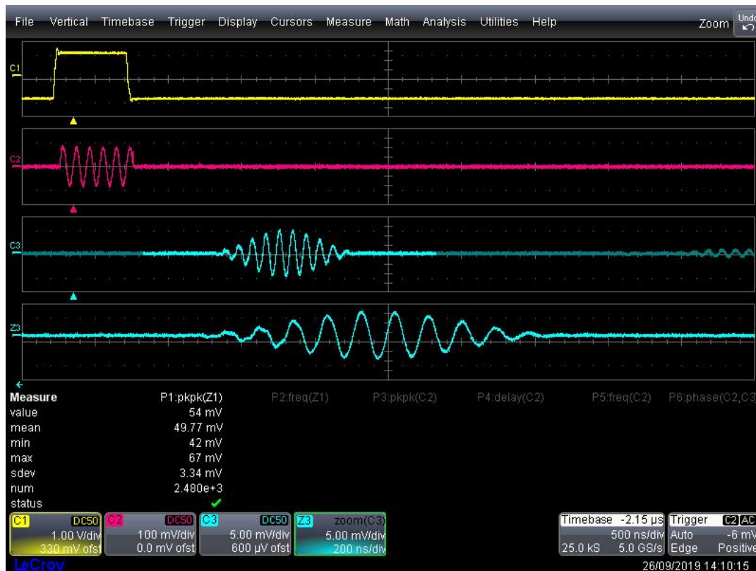
FIGURE 4.12: A screenshot from a typical SAW measurement taken by the oscilloscope system. Channel 1 (C1) is the pulse signal, Channel 2 (C2) is the input reference signal, Channel 3 (C3) is the output signal from the SAW device and Z3 is a zoomed section of C3.
