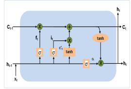
Figure 2. Structure of LSTM Unit.
