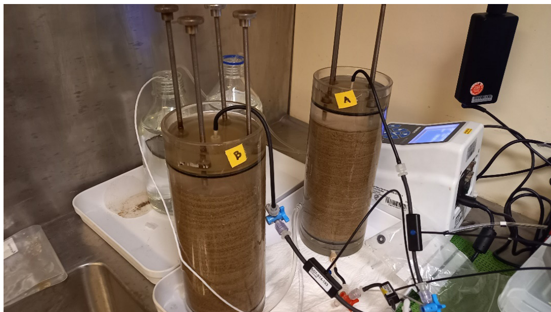
Fig. 12.2: Flow through reactor set-up: Flow through cells for determining oxygen concentrations can be seen at the upper and lower inlets of the reactors.
