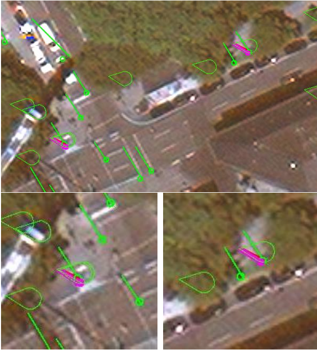
Figure 17. top: section 60 \times 36 \text{ m}^2 of fig. 15 (NE of center, Maximiliansplatz), bottom: details ( 20 \times 20 \text{ m}^2 ) with determined corrections as pink lines from pole footpoint to SAR-GCP
