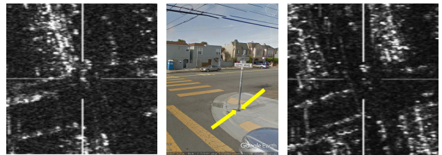
Figure 5. Example of a SAR measurement (Lawton Street, San Francisco), left TerraSAR-X image from 2017-04-12, center Street-View image (© Google) with TerraSAR-X acquisition directions, right TerraSAR-X image from 2017-04-15, pole in the center of the TerraSAR-X images
