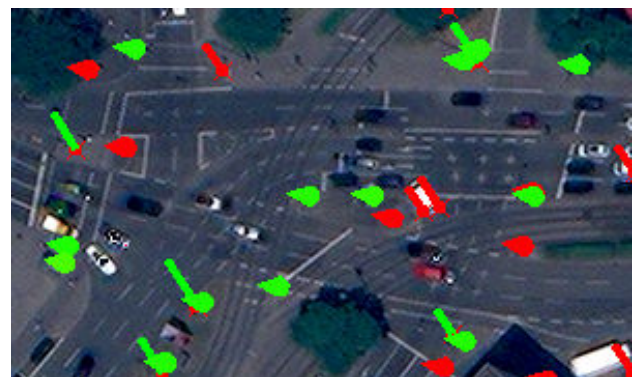
Figure 19. Detail 90 \times 54 \text{ m}^2 of fig. 18 showing correct detected poles and GCPs in green and misdetections in red
