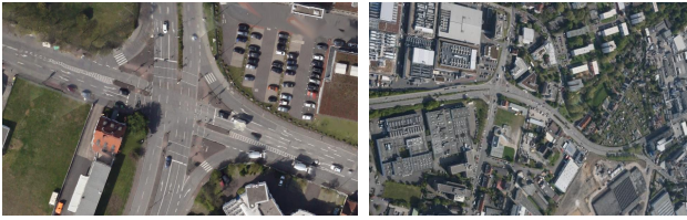
Figure 2. Crossing “Am Seedamm/Eschborner Landstraße” in Frankfurt am Main (Germany), left: aerial ortho image 150 \times 90 \text{ m}^2 , GSD 15 cm, right: original right looking image containing the crossing (south is right)
