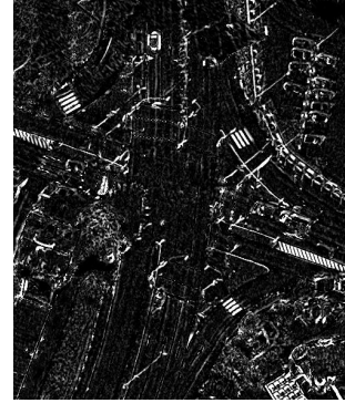
Figure 9. Same section as in fig. 8, result after filtering narrow objects relatively darker than their surrounding (shown in white)
