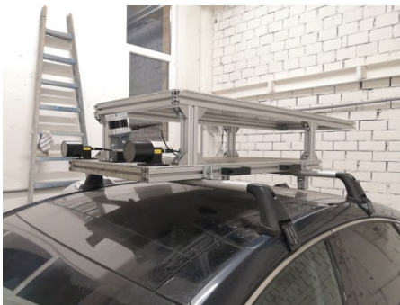
(a) Placement of stereo camera, inertial sensor and LIDAR.
