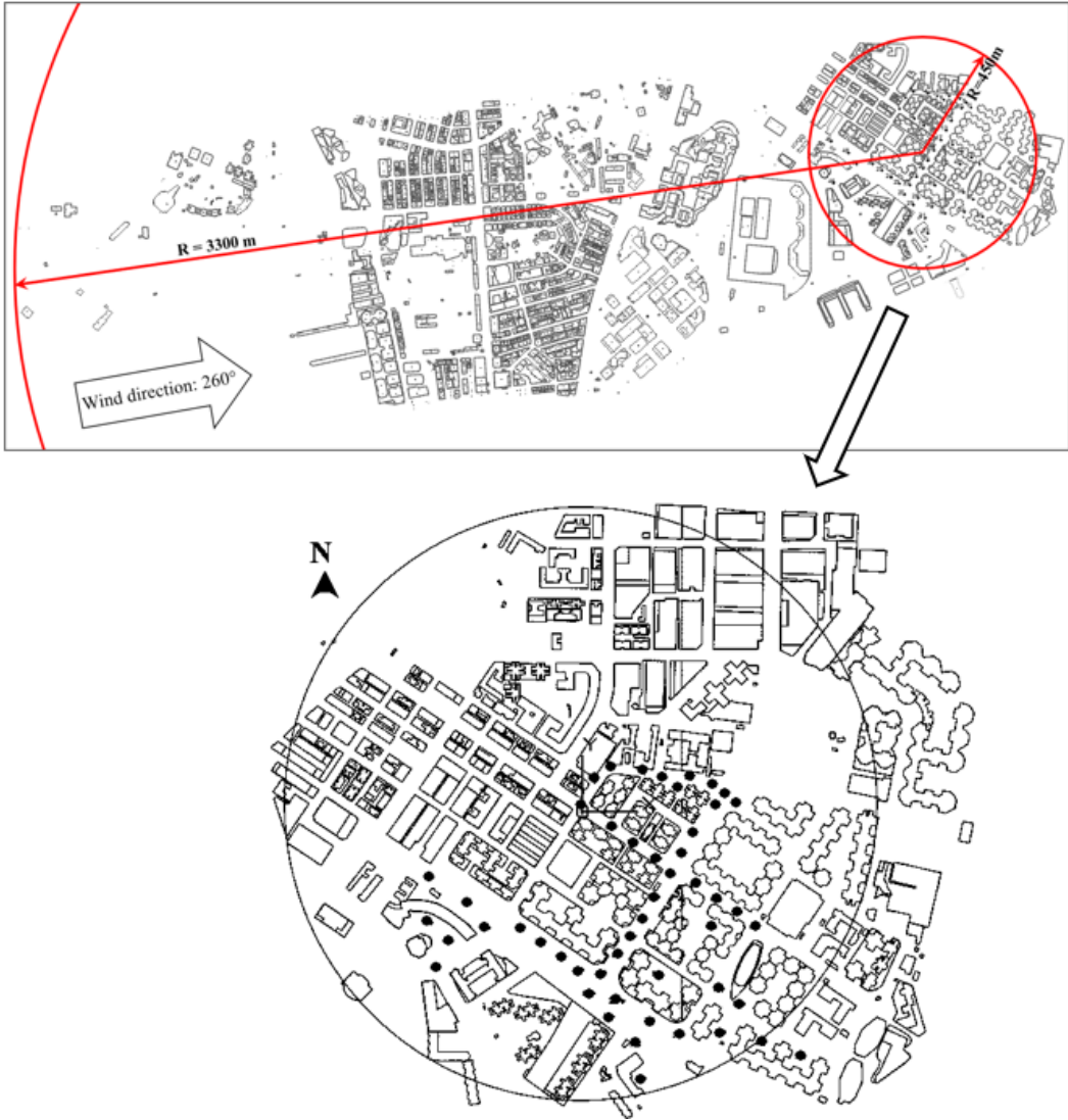
Figure 6.7 Critical wind direction and observation points.
