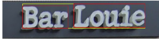
Figure 4.10: A sample from the word-level annotation CSV file and its representation on the image where yellow bounding box surrounds the full text patch and the red ones show the annotation at word-level.
