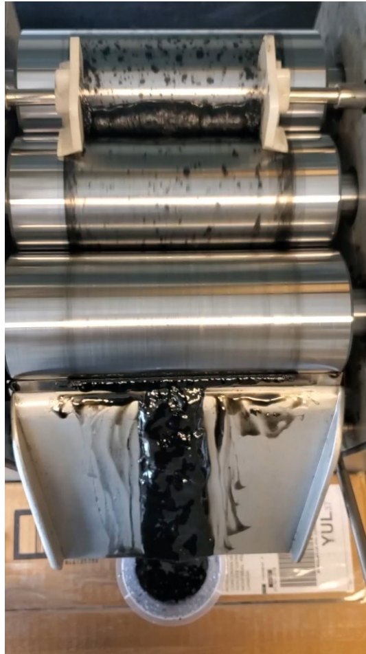
Figure 19: CNTs being dispersed in epoxy resin using three roll milling
