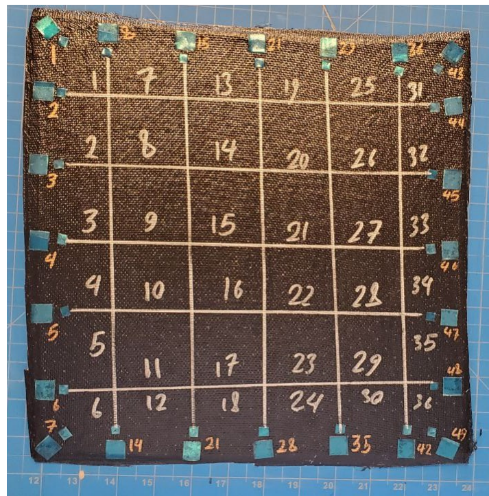
Figure 29: A cured sample with node numbers on the edges and cell numbers in the middle of each cell
