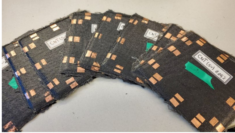
Figure 21: Samples made with different concentrations of CNT
