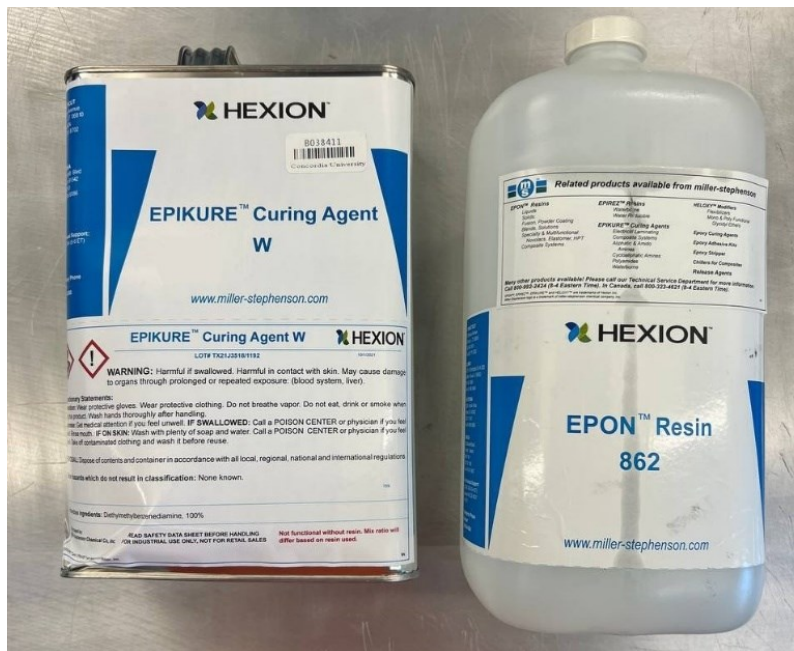
Figure 17: Epoxy resin and Curing Agent used to prepare samples
