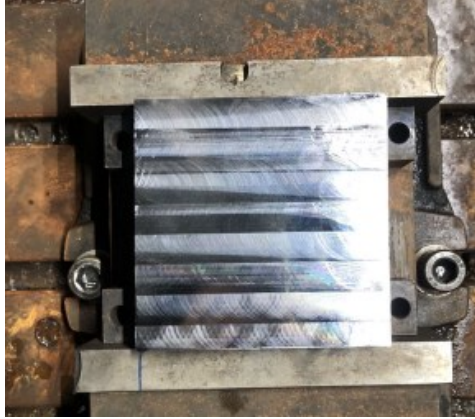
Figure 2.26 The 2Cr13 stainless steel workpiece is fixed in a vise.
