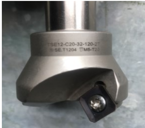
Figure 2.24 The TSE12 indexable face mill has two inserts.
