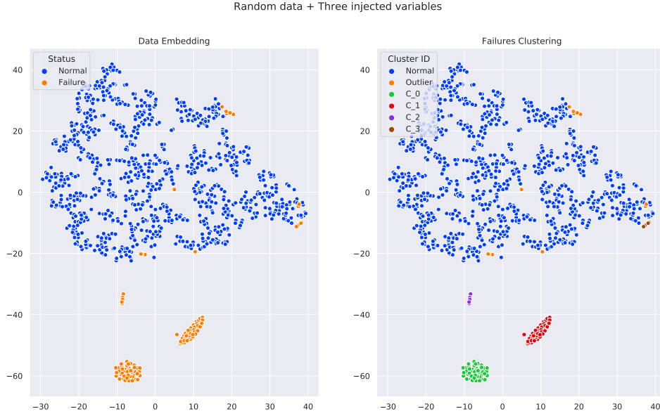
Figure 8: Normal and Failure samples in the embedding space of \mathcal{S}_2 . The data is generated from i.i.d. random uniform distributions except for 3 columns, which associated with Failure samples. There are 4 clusters for Failure samples.
