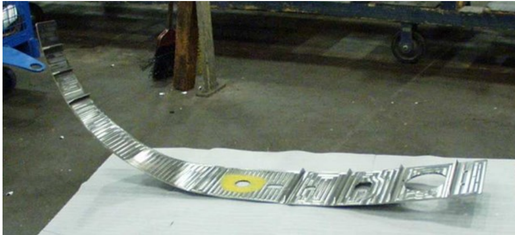
Figure 1.6 Flat machined airframe component distorted due to residual stress
