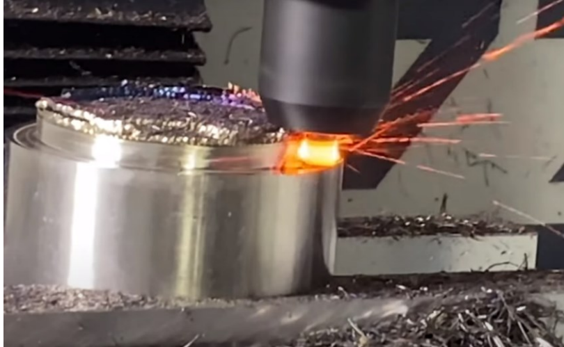
Figure 1.5 Continuous chips and high temperature in the milling of Inconel 718
