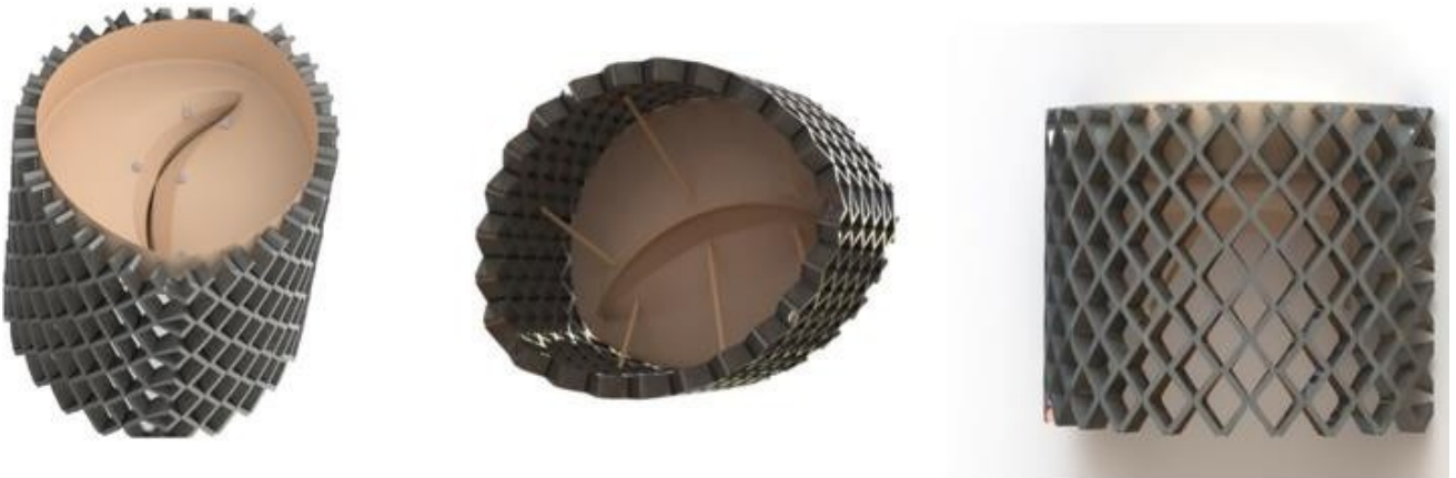
Figure 3-7. Mitral valve CAD drawing including the artificial chordae tendineae
