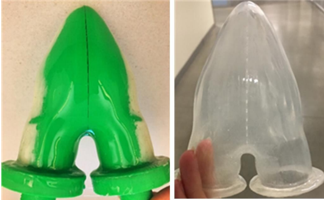
Figure 3-1. Left ventricle mold before and after taking off the silicone
