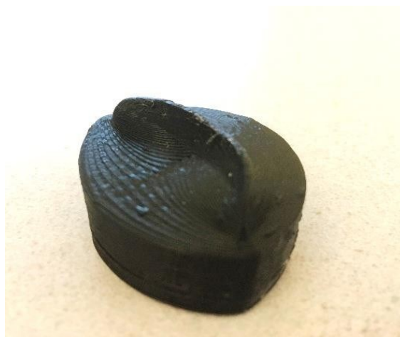
Figure 3-6. 3D printed mitral valve leaflets mold, printed by a FDM printer, Lulzbot Taz 6, with a PLA filament
