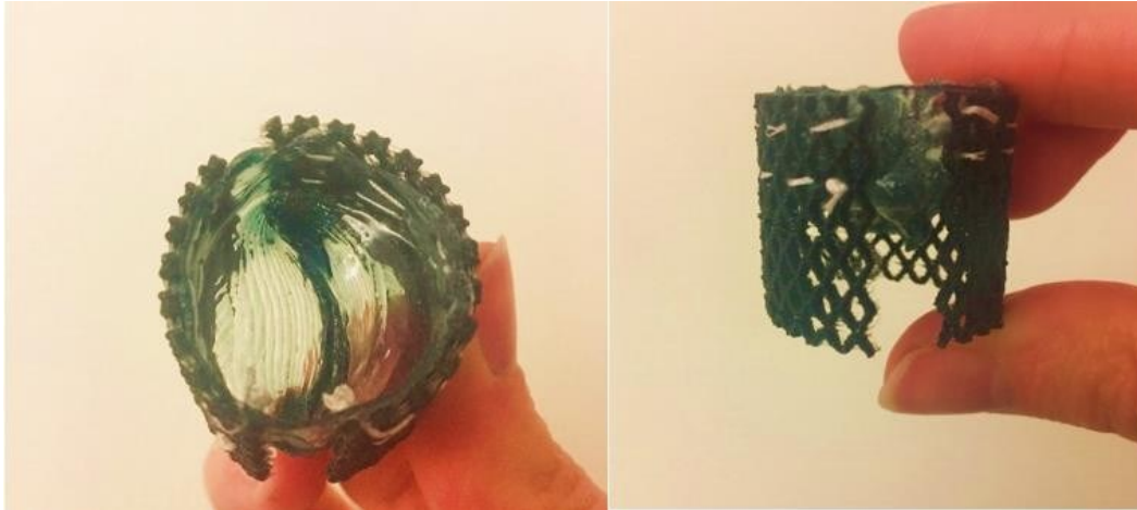
Figure 3-8. Mitral valve before attaching the artificial chordae tendineae
