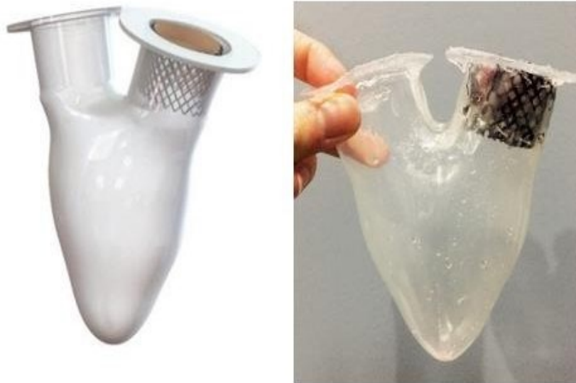
Figure 3-9. Placement of mitral valve in the left ventricle
