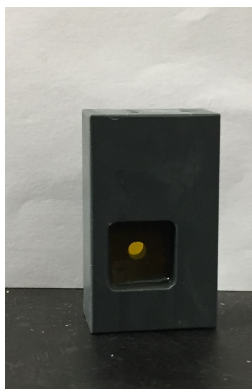
Figure 1.26: Sample chamber for our in-house source at LMU. Sample is filled with a pipette through a small hole in the top. Kapton is glued to the plastic chamber.
