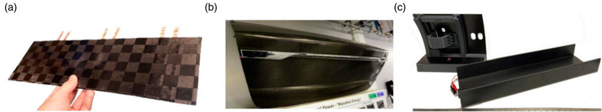
Figure 2. Previous structural power demonstrators (a) panel with integrated SBCs 15 ; (b) Volvo boot lid with integrated SSCs 7 ; (c) fuselage rib with integrated SSCs. 16
