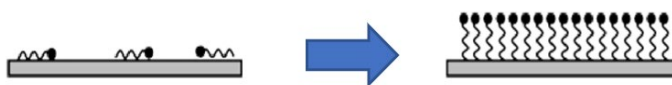
Figure 2. 20 Illustration of adsorption of surfactants at a hydrophobic surface for a) low and b) high concentrations 143 .
