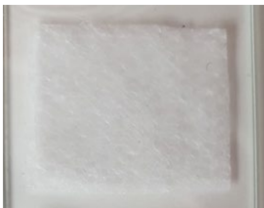
Figure 4. 7 Polyolefin based nonwoven, (2x3cm) fixed into a microscope slide using double sided tape.
