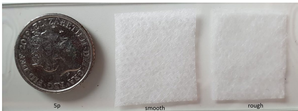
Figure 4. 10 Photo showing the “smooth” and the “rough” surface sides of a typical nonwoven. Note the 5p is included illustrative purposes to give an idea of the size of these patterns.
