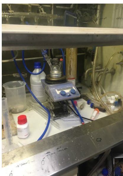
FIGURE 2.6: PHOTOGRAPH OF THE EXPERIMENTAL SET-UP FOR THE THERMAL DECOMPOSITION OF IRON ACETYLACETONATE UNDER NITROGEN.
