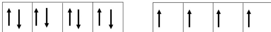
FIGURE 1.10: ILLUSTRATION OF THE ELECTRONIC STRUCTURE OF A DIAMAGNETIC MATERIAL (L) AND A PARAMAGNETIC MATERIAL (R)
