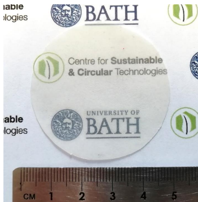
Figure 4. Photograph of the film produced from poly(2a)-H (diam. 50 mm, thickness 170 \mu\text{m} ).
