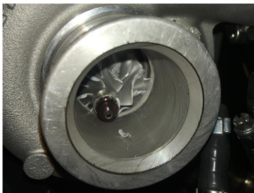
Fig. 11. Turbocharger failure as a result of testing at 135 krpm.
