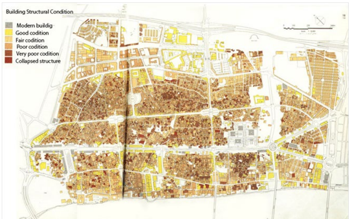
Figure 6: The Area of Old Rusafa, Building Structural Condition Source: (JCP 1984).
