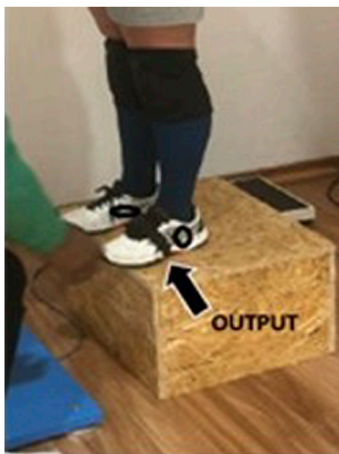
FIGURE 3 OUTPUT mobile inertial unit and the positioning strap.
