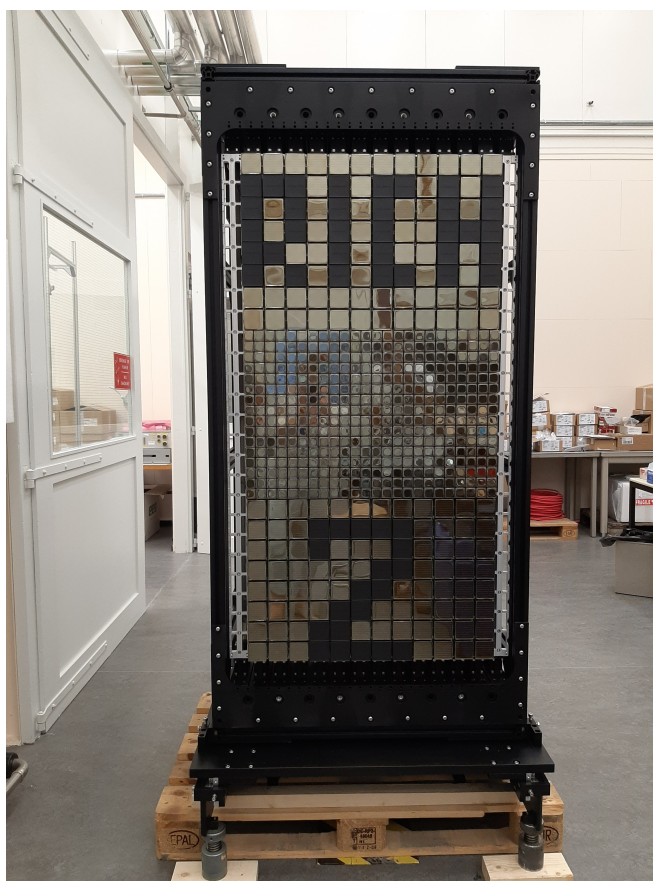
Figure 4.11 Photograph of RICH2 A-side columns ready to be installed into the LHCb detector. The 2x2 inch MaPMTs are on the outside regions and the 1x1 inch are on the central regions of the detector.
